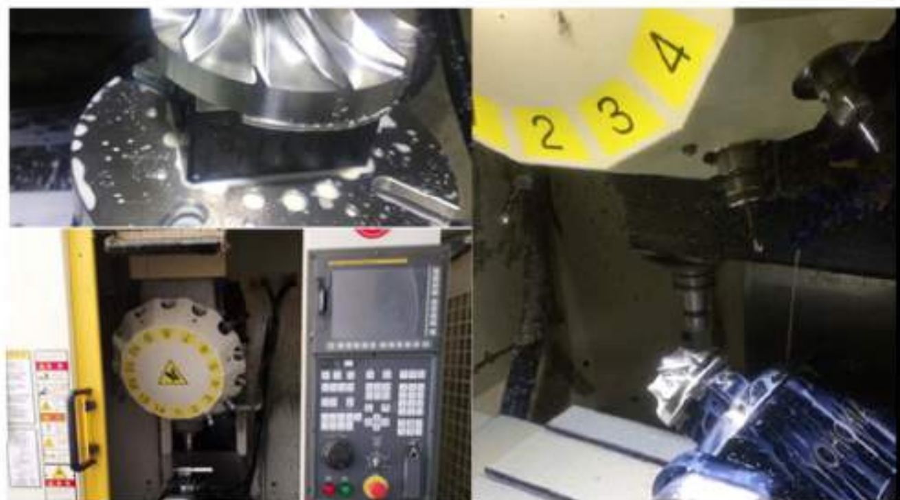
叶轮加工 (小黄机FANUC 31i+YHM160H五轴转台) Impeller processing (Xiaohuang machine FANUC 31i+YHM160H five-axis turntable)
