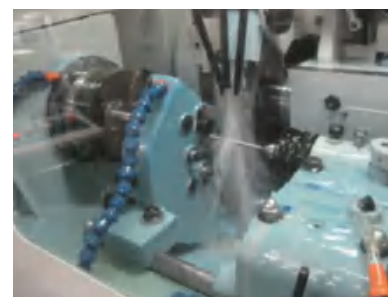
通过螺纹磨床进行的高精度螺纹槽加工 High accurate shaft groove process by Grinding machine
